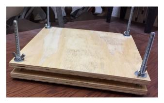
**Summary:** You will drill holes in two flat piece of wood and use screws and wing nuts to make a press.
