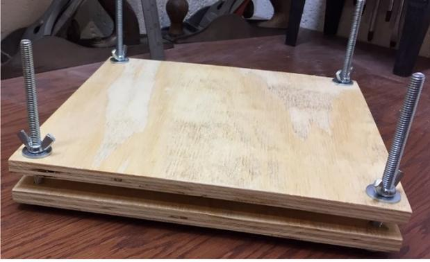
**Summary:** You will drill holes in two flat piece of wood and use screws and wing nuts to make a press.
